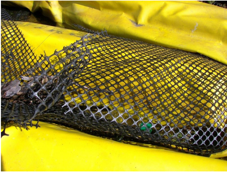
Figure 10: Pre-2009 Damaged Milfoil Fragment Barrier – when barriers blocked access.
