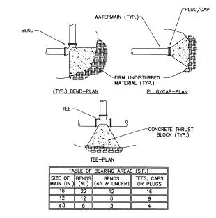
NOTES: 1. CONCRETE FOR THRUST BLOCKS SHALL HAVE MINIMUM COMPRESSIVE STRENGTH OF 2000 PSI AT 28 DAYS, UNLESS DIRECTED OTHERMISE BY THE ENGINEER OR OWNER
