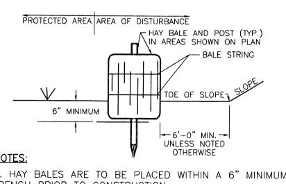
1. HAY BALES ARE TO BE PLACED WITHIN A 6" MINIMUM TRENCH PRIOR TO CONSTRUCTION.
