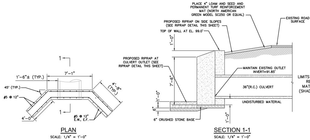
**PROPOSED CAST-IN-PLACE HEAD & WING WALLS**
