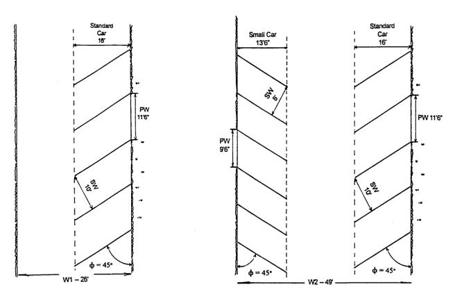
PW=SW / sine W1 & W2 are wall to wall layouts. If parking is curb to curb, subtract 1 ft. - 6 in. from table dimensions for W1, and 2 ft. for W2.
