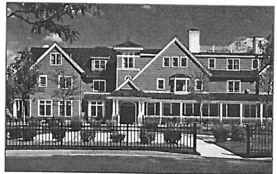
Figure 97: A larger building façade is broken into vertical and horizontal patterns with a balanced rhythm
