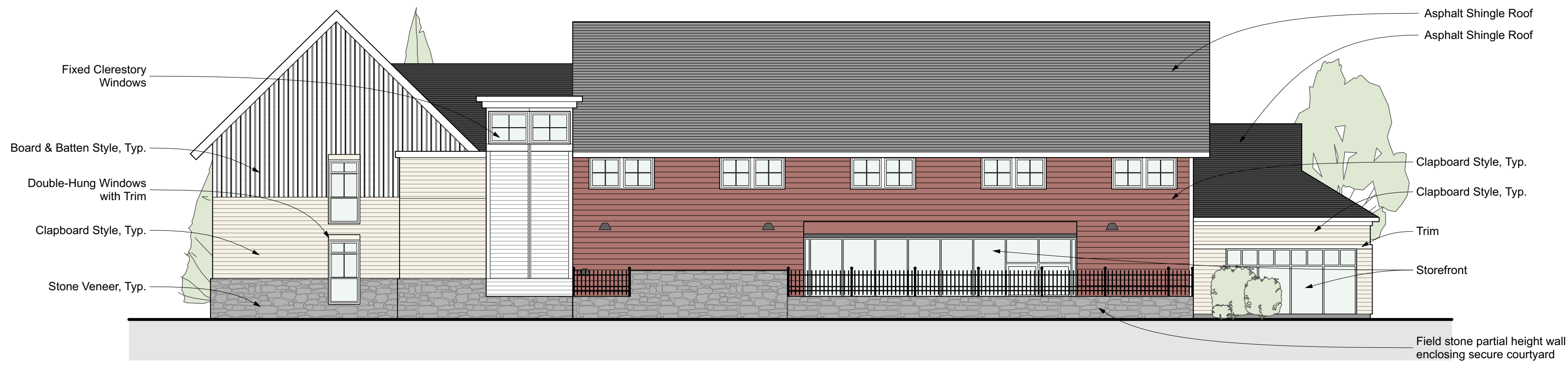
1 NORTH ELEVATION FROM STREET Scale: 3/32" = 1'-0"
