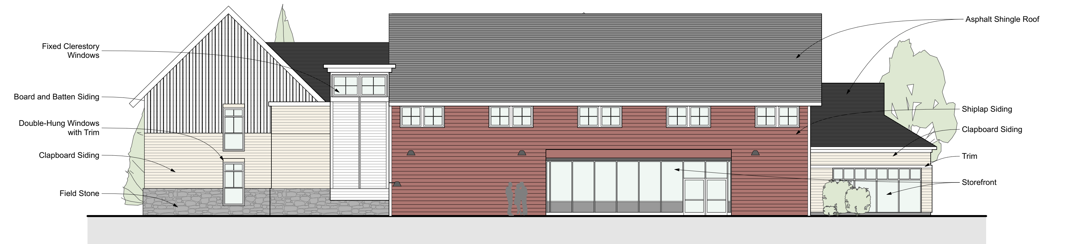
2 NORTH ELEVATION FROM SECURE COURT Scale: 3/32" = 1'-0"
