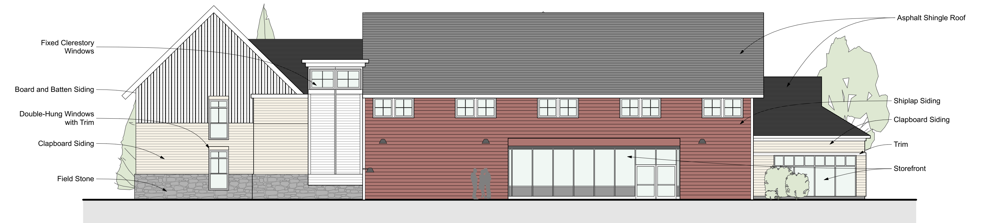
3 NORTH ELEVATION FROM SECURE COURT Scale: 3/32" = 1'-0"
