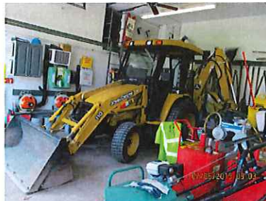
Parks and Recreation's John Deere Excavator: backhoe, bucket loader, auger and brush attachments. A brush hog can be added.
