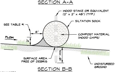
INSTALLATION NOTES: I. INSTALL SILT SOCK ON A SURFACE CLEAR OF DEBRIS.
