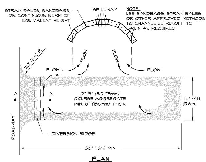
I. THE ENTRANCE SHALL BE MAINTAINED IN A CONDITION THAT WILL PREVENT TRACKING OR FLOWING OF SEDIMENT ONTO PUBLIC RIGHT-OF-WAYS. THIS MAY REQUIRE TOP DRESSING, REPAIR AND/OR CLEANOUT OF ANY MEASURES USED TO TRAP SEDIMENT.
