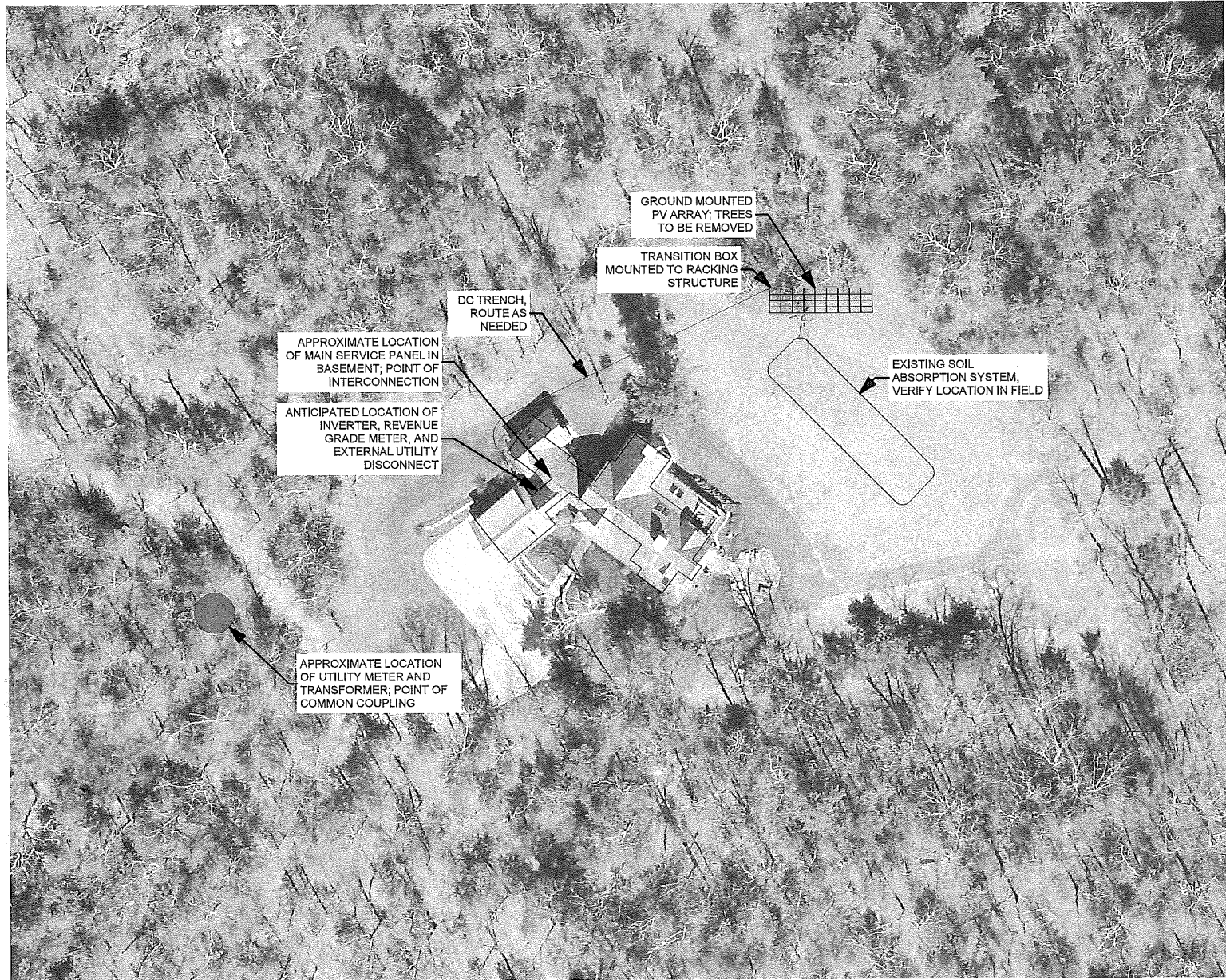
1 9.18 KW DC (10 KW AC) PV ARRAY WITH (36) 255W MODULES AT FIXED 25 DEGREE TILT 0 16' 32' 64'
